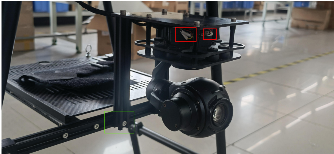
平台安装后，安装云台吊舱，螺丝对应螺母及垫片的安装锁紧方式；After the platform is installed, install the gimbal pod and lock the screws with corresponding nuts and washers.
